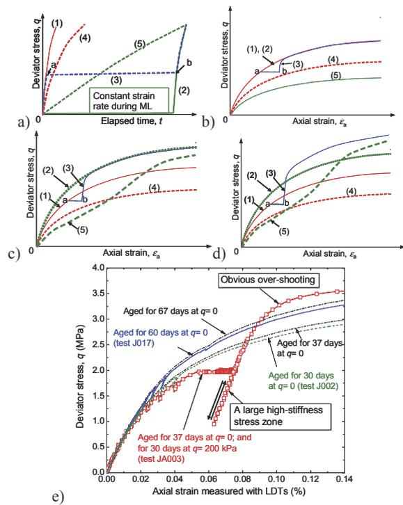
Fig. 16.2. a) Various loading histories in drained TC; and stress-strain curves for elasto-viscoplastic models; b) without ageing; c) with ageing (no coupling); and d) with ageing (positive coupling); and e) drained TC tests on moist cement-mixed gravelly soil ( $\sigma'_c = 19.7$  kPa &  $d\epsilon_v/dt = 0.03$  %/min) (Kongsukprasert & Tatsuoka, 2005).
