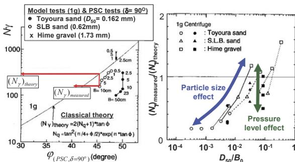
Fig. 9.2. Particle size effects on  $N_\gamma$  for a strip footing on a granular material (Tatsuoka et al., 1997).
