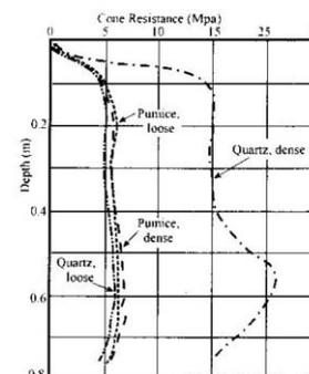
Fig. 6.2. Typical CPT Results for Pumice & Quartz Sands
