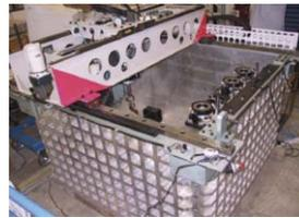
Fig. 10.1.1. The 4-axis robotic manipulator at HKUST (Ng et al. 2002b)
