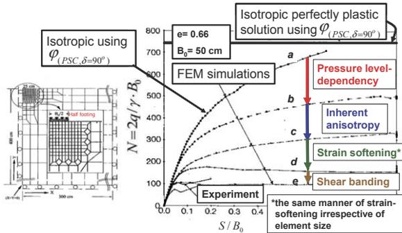
Fig. 16.1. Effects of assumptions in the constitutive model for sand on the plane strain FEM analysis of the bearing capacity of a strip footing on Toyoura sand (Siddiquee et al., 1999).
