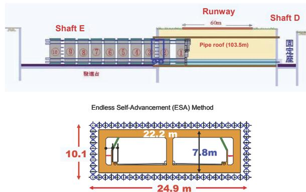
Fig. 10.3.2. Construction sequence
