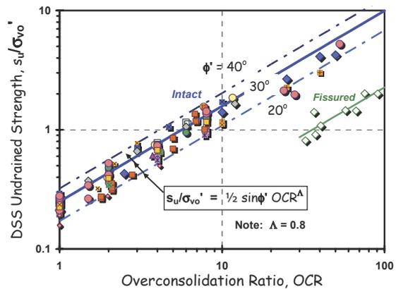
Figure 7.2. CSSM undrained strengths for OC clays (Mayne 2005).
