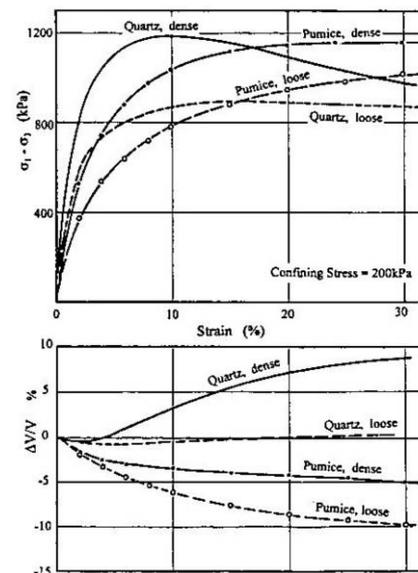
Fig. 6.1. Typical Triaxial Behaviour of Pumice & Quartz Sands
