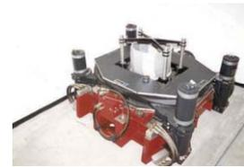
Fig. 10.1.2. The bi-axial shaking table at HKUST (Ng et al. 2004)
