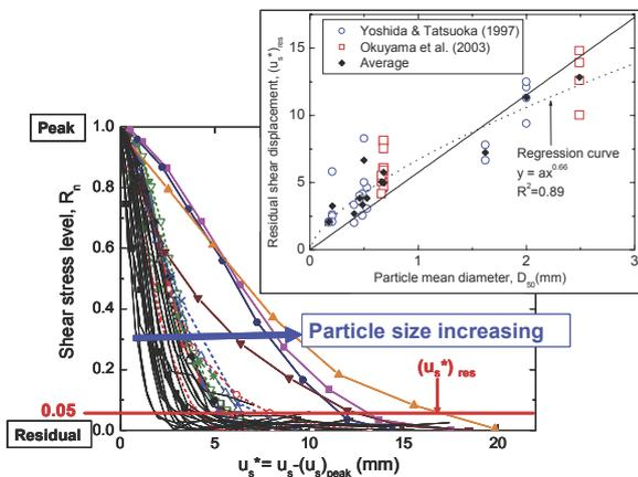
Fig. 9.1. Effects of particle size on the shear deformation of shear band in drained PSC tests (Okuyama et al., 2003).
