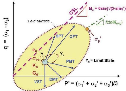
Figure 14.2. Conceptual Stress Paths for Various In-Situ Tests
