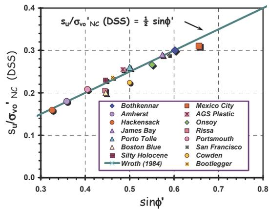
Figure 7.1. CSSM-evaluated undrained strength at OCR = 1.
