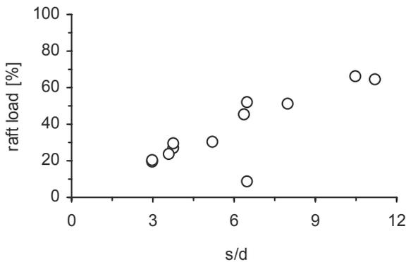
Fig. 10.2.1. Experimental evidence of load sharing between raft and piles. 11 case histories with piles uniformly spread over the whole foundation area
