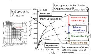
Fig.16.1. Effects of assumptions in the constitutive model for sand on the plane strain FEM analysis of the bearing capacity of a strip footing on Toyoura sand (Siddiquee et al., 1999).
