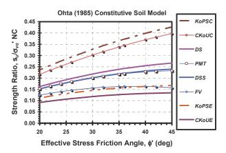
Figure 14.1. Hierarchy of undrained strength modes for NC clays using CSSM model with rotated bullet yield surface (after Ohta, et al. 1985).
