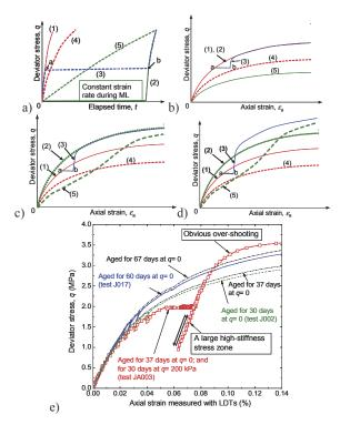
Fig. 16.2 .a) Various loading histories in drained TC; and stress-strain curves for elasto-viscoplastic models; b) without ageing; c) with ageing (no coupling); and d) with ageing (positive coupling); and e) drained TC tests on moist cement-mixed gravelly soil ( $\sigma'_c$ = 19.7 kPa & de<sub>v</sub>/dt= 0.03 %/min) (Kongsukprasert & Tatsuoka, 2005).
