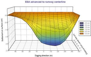
Fig. 10.3.3. 3-D Settlement prediction before construction
