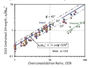
Figure 7.2. CSSM undrained strengths for OC clays (Mayne 2005).
